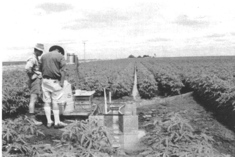
Figure 1. Instrumentation installed at plot-scale in central Queensland for measuring and sampling runoff
