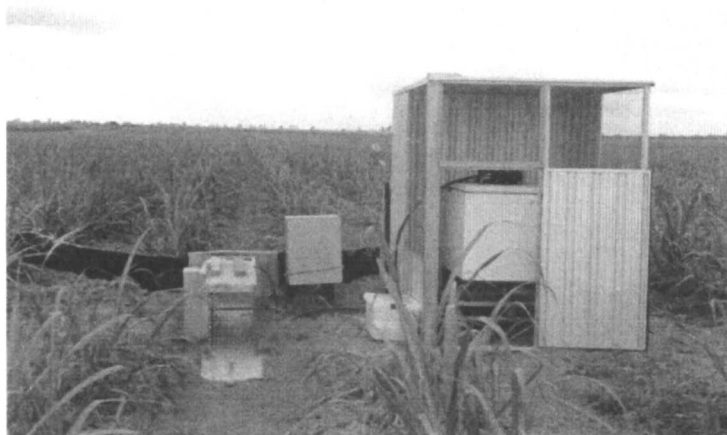
Figure 4. Instrumentation at plot-scale (SE Queensland) for measuring and sampling runoff
