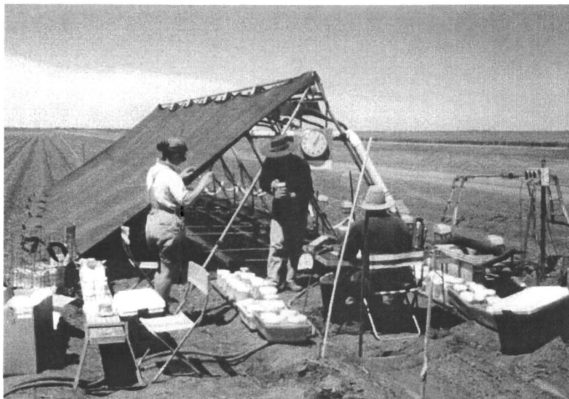
Figure 4. Rainfall simulator on two cotton furrow plots, with sample bottles laid out for runoff and sediment, sediment size and pesticide runoff (6).
